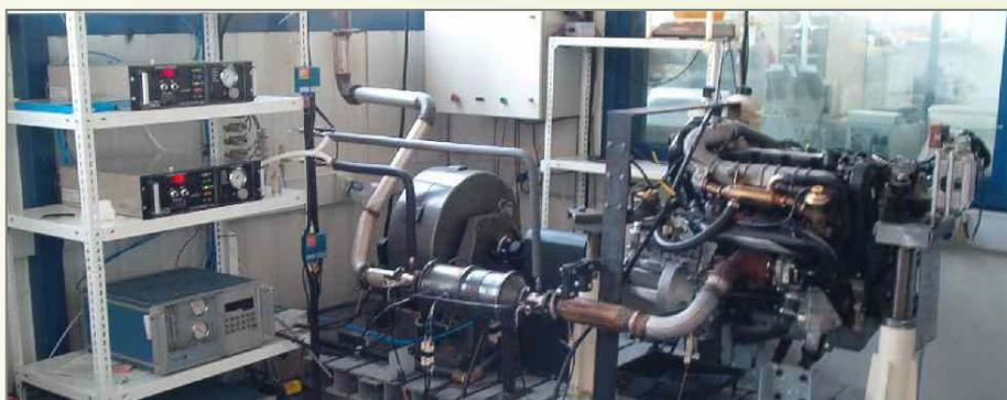
Internal combustion engine test bed
